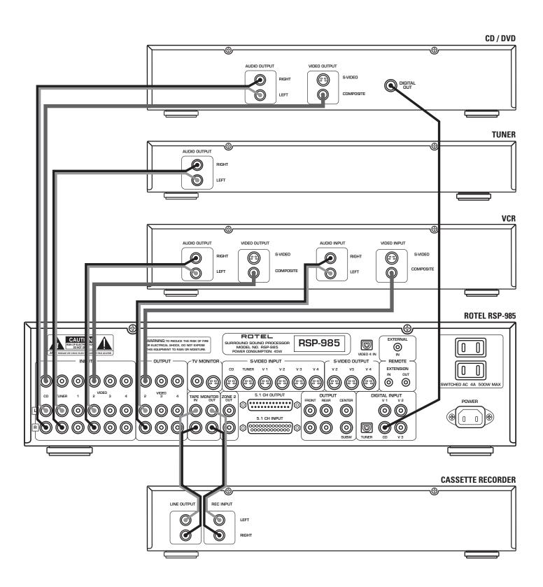
Figure 5 - S-Video Source Connections
